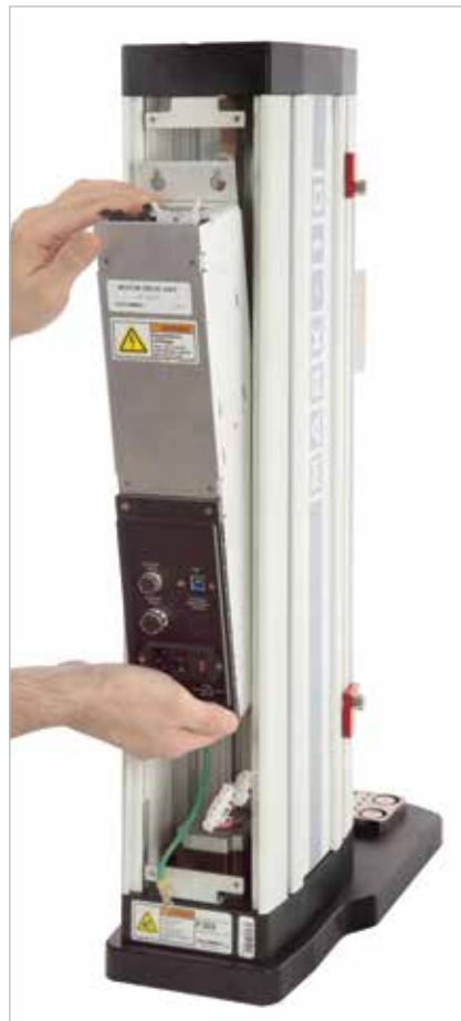
Removing the electronics module
