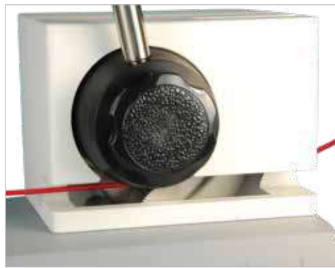
▲ Unique knurled cam design effectively secures and pulls the loose end of the sample.
