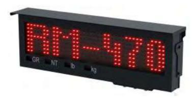
Powder coated steel housing which includes a drop-down electronics carriage for quick and easy installation and service. 8x40 pixels, 4.7" full matrix LED boards allow to display Gross/Net/Tare indicators. Easily visible from up to 170 feet.
