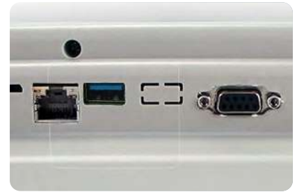
RS-232, USB or optional ethernet, Wi-Fi or Bluetooth connectivity
