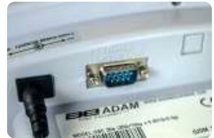
RS-232 interface provides speedy connection to computers and printers
