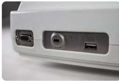
USB-A and RS-232 interfaces provide speedy communication with computers
