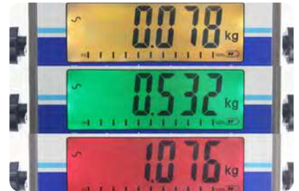
Color-changing backlight for easier checkweighing
