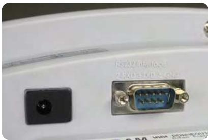
RS-232 interface for sending data to PCs and printers
