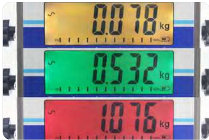
Display backlight changes color during checkweighing
