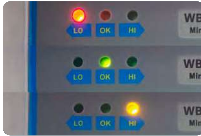
Checkweighing LEDs clearly show under, over and within acceptable limits
