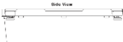
Bracket to hold polyethylene top deck when cleaning under scale
