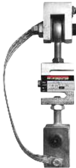
Module with RL200001 S-beam load cell
